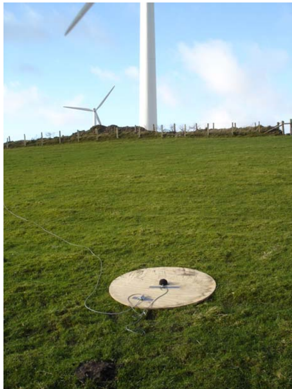
Figure 4 (Left) Standard measurement setup with ground board.
