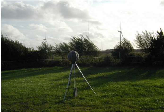
Figure 29 Noise monitoring position at Neighbour to Høvsøre Test Site.
