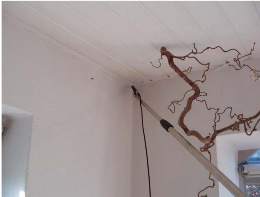
Figure 6 Example of a 3D position with the microphone placed in the three-dimensional corner where two walls and the ceiling meet.
